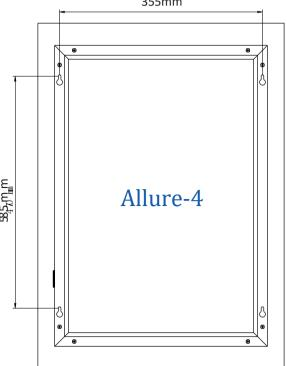
The drawing above shows the dimensions for wall drillings for the installation of the mirror
