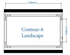
Following the relevant diagram for your mirror mark the 4 hanging positions onto your wall.
